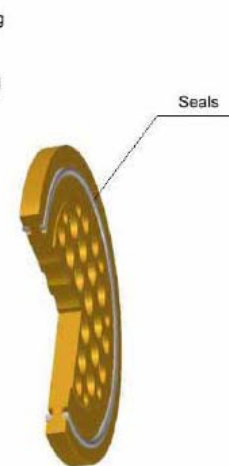
Figure 3 Zanker Board-type Flow Conditioner
